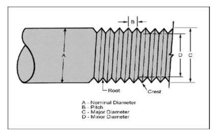
In the above figure, the arrows point to the root and the crest of the threads. The pitch of the thread is the distance from the crest of one thread to the crest of the next thread. This measurement is used to determine the number of threads per inch, or millimeters per thread, data that are usually supplied by the fastener manufacturer. The one most frequently used term in designating the size of a bolt or screw fastener is its nominal diameter.
