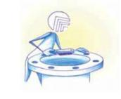
Examine the flange surfaces, fasteners (bolts or studs), nuts and washers to ensure they do not have any serious defects. Replace any components if found to be defective. If in doubt, seek advice from a qualified expert.
