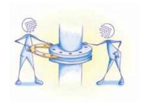
Bring the flanges together ensuring the gasket is not pinched or damaged.
