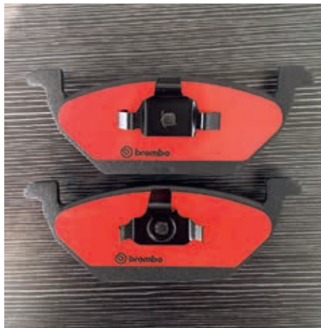
RCM employed as a shim on disk brake pads
