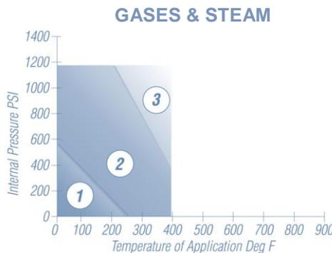
In area ①, the gasket material is suitable using common installation practices subject to chemical compatibility.
